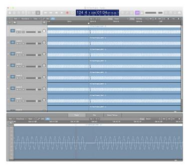
A T2 audio glitch captured during recording. The entire waveform should be smooth and uninterrupted. Some glitches like this could probably be edited, but errors like these can destroy a recording.
