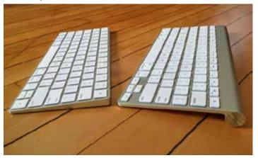
Perhaps most significantly, the back edge of the keyboard doesn't rest atop a cylinder running the full length of the keyboard, which was a necessary element on the old keyboard to accommodate the battery compartment. The power button is now a toggle switch on the back instead of a round button at one end of the old cylinder.
