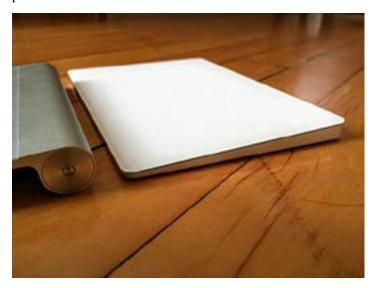
The Magic Trackpad 2, like the Magic Keyboard, is a simpler, slightly tilted platform with toggle-style power switch on the back. The two line up reasonably well, though not perfectly since the trackpad's upper surface is, oddly, a bit taller than that of the keyboard. That annoys some people and seems like a major gaffe from Apple's vaunted industrial design teams.
