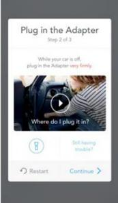
To install the Automatic Link, you need to plug it into a gasoline-powered car with an OBD-II port, which is common to cars from model year 1996 and later. You can usually find this port between the steering wheel and pedals. When prompted by the app, plug the Link firmly into this port — it's reminiscent of inserting a cartridge into an old video game console. Once installed, the Link is hard to notice, so don't worry about it attracting opportunistic thieves.
