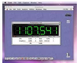
In other words, a Mac Pro which would otherwise be double the speed of a G5 ends up running SheepShaver at less than one-tenth the CPU speed. The only bright spot found here is in the Math score, which remains the same between the G5 and the Mac Pro.
