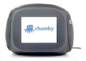
**Chumby 101** — So what the heck is a Chumby, anyway? Take a beanbag about the size of a grapefruit and stuff it with a 3.5" color LCD touch screen, a 350 MHz CPU, 128 MB of memory, Wi-Fi, a motion sensor, a squeeze sensor, two USB ports, a pair of speakers (and headphone jack) and you have a Chumby.
